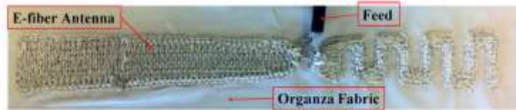
Fig. 1-22 Embroidered textile AMF antenna on organza fabric [65]
