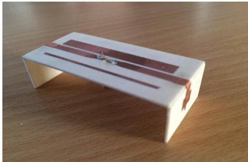
*Fig. 2-3 Fabricated 3-D antenna*
