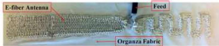
*Fig. 1-22 Embroidered textile AMF antenna on organza fabric [65]*
