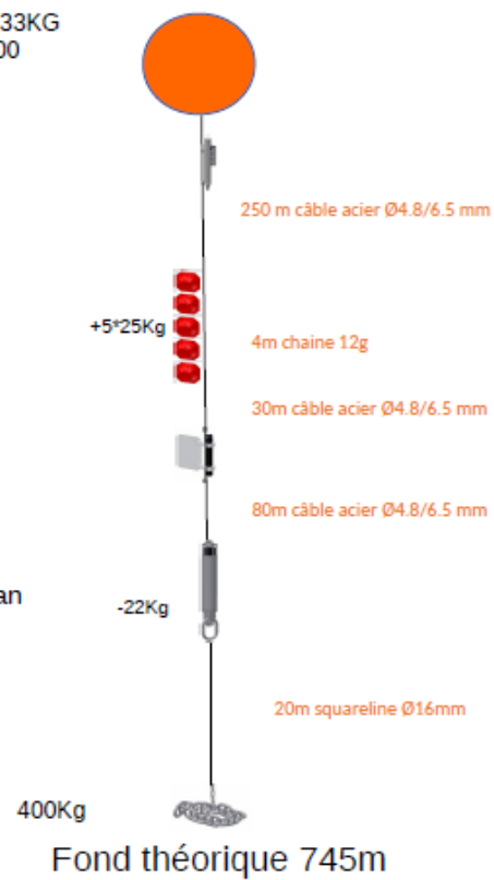
Figure 4.1: Schematic of the mooring that will be deployed this summer in the Yermak Pass
