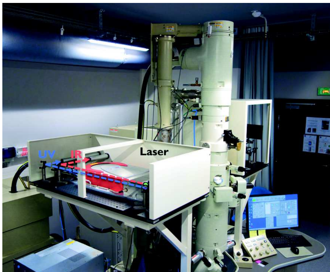
Figure 4.1: Photo showing the UTEM in Strasbourg. The left optical table contains the laser head with the UV module.
