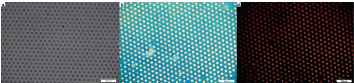
Figure 2. 7 (a) Optical microscopic image of the PDMS stamps used for \mu CP experiments. 21 \mu m circular (b) Optical microscopic images of a 21 \mu m sized pattern of a dewetted PS film on a Si/SiO 2 patterned substrate. (c) A contrasted optical microscopic images of a 21 \mu m sized pattern of a dewetted PS film on a Si/SiO 2 patterned substrate.
