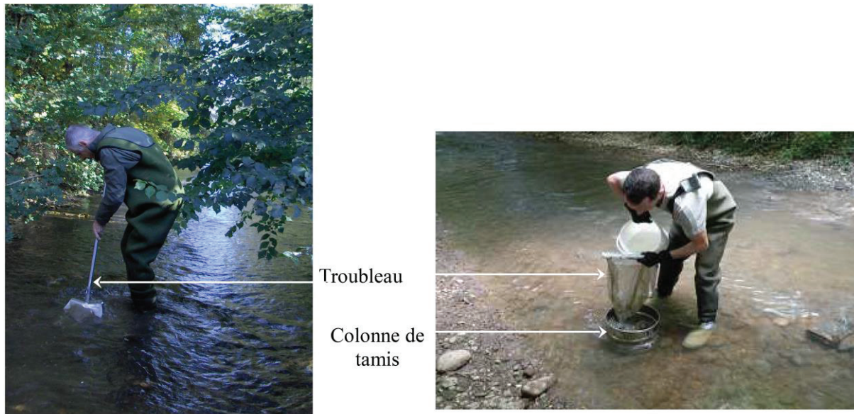
Figure II-2 – Organism collection using the fishnet and the sieve.
