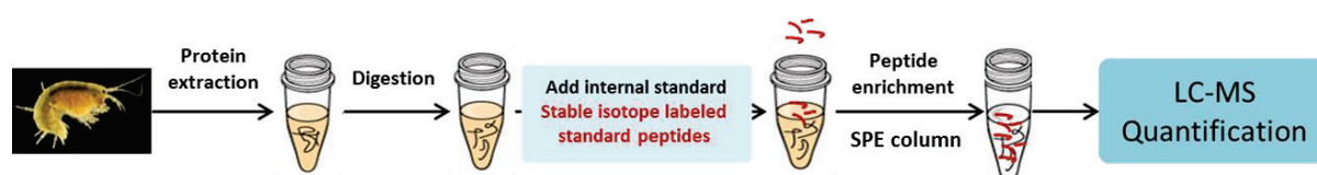
Figure II-10 – Main stages of sample preparation for SRM analysis. SPE – solid phase extraction.
