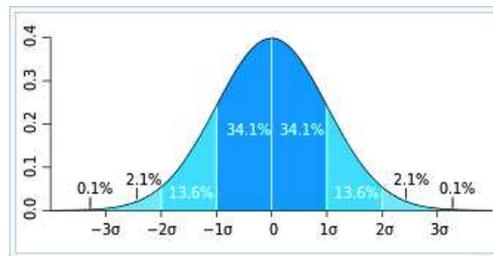
Figure 3.2 – From Wikipedia: A reminder about the standard deviation  $\sigma$  and the stochastic meaning  $\pm 2\sigma$  and  $\pm 3\sigma$  intervals [To be used when interpreting the results in Figure 3.1]. Recall: 68% of the data lie within 1 standard deviation, 95% within 2 and 99.7% within 3.
