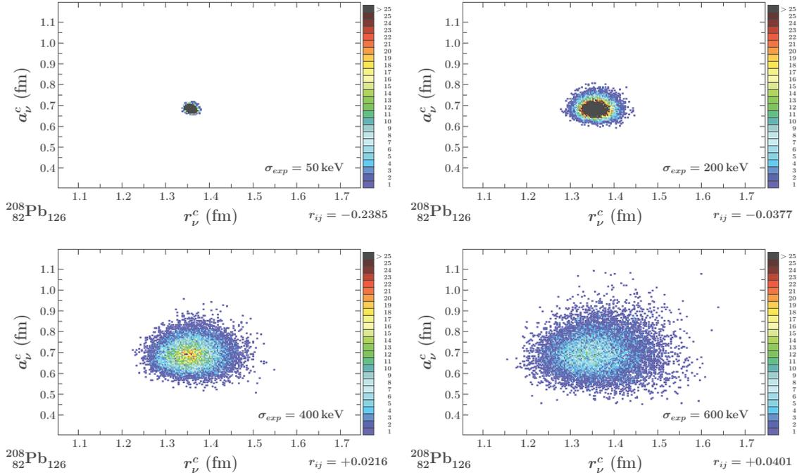
Figure 4.7 – Similar to the preceding one but for the neutron central radius  $r_\nu^c$  and central diffuseness  $a_\nu^c$  in  $^{208}\text{Pb}$ . As before, the radial symmetry of the diagrams suggests that the parameters are uncorrelated and the small values of the Pearson coefficient confirm this.
