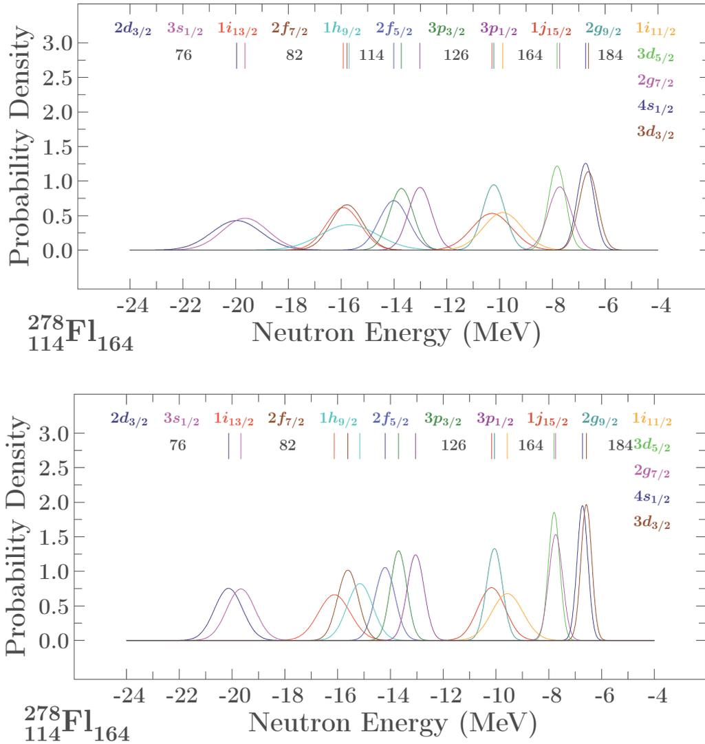
Figure 4.23 – Neutron probability density distributions for  $^{278}\text{Fl}$  fitting with full parametric freedom (top) and after full parametric correlation removal, imposing compact spin-orbit solution (bottom). The values of the corresponding FWHM can be found in Tables 4.7 and 4.17 for top and bottom results, respectively.
