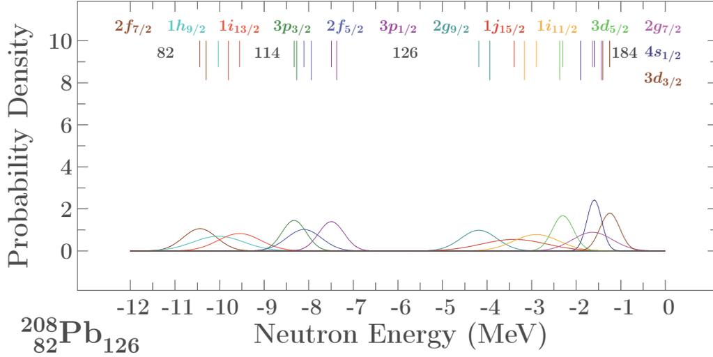
Figure 5.9 – Uncertainty probability distributions for the neutron single particle energies within the main nuclear shells  $N_{\text{main}} = 5$  and 6. They have been obtained using realistic Monte Carlo simulations with  $\sigma_{exp} = 600$  keV using the density-dependent spin-orbit and minimising over the set of parameters in Eq. (5.21), keeping  $a_{\pi}^c = a_{\nu}^c = 0.7$  fm. The FWHM of each distribution can be found in Table 5.3. The surface under each curve is equal to 1.
