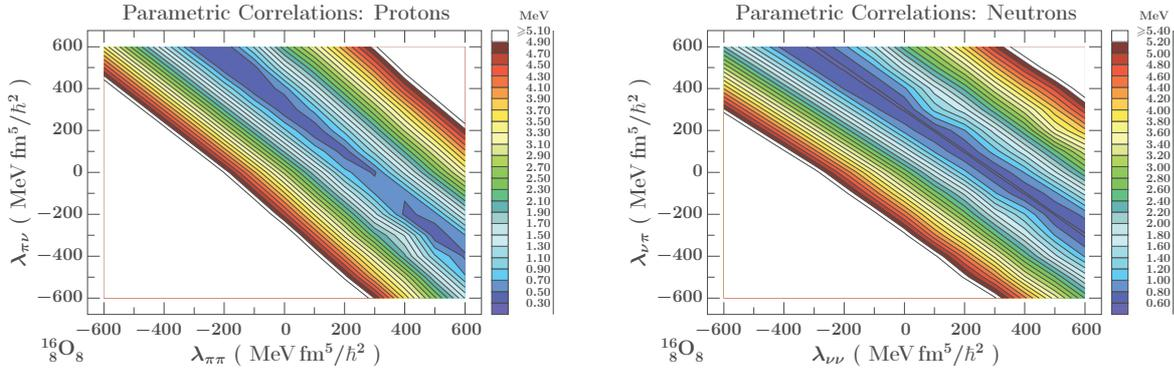
Figure 5.23 – Left: Proton r.m.s.-deviation in MeV projected onto the  $(\lambda_{\pi\pi}, \lambda_{\pi\nu})$ -plane for  $^{16}\text{O}$  nucleus. The central potential parameters were kept fixed at the optimal values for  $^{16}\text{O}$ . At each  $(\lambda_{\pi\pi}, \lambda_{\pi\nu})$  value the  $\chi^2$  was minimised over  $\lambda_{\nu\nu}$  and  $\lambda_{\nu\pi}$ . The colour scale gives the proton-r.m.s. deviation in MeV. Right: Analogous illustration for the neutrons.
