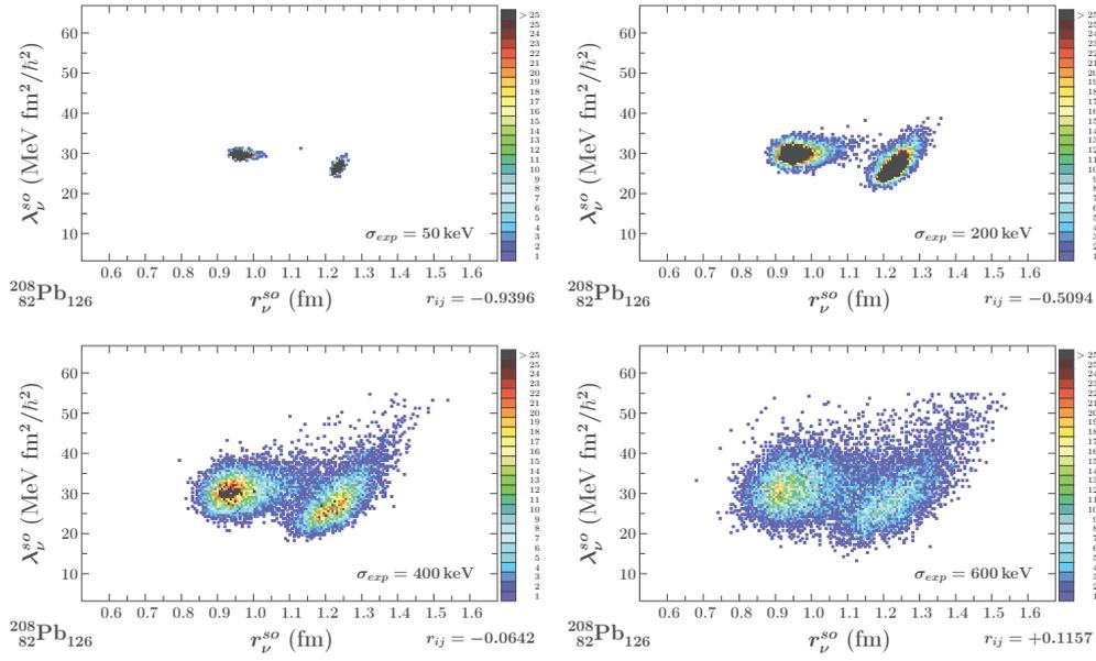
Figure 4.13 – Parametric correlation between the neutron spin-orbit radius  $r_n^{so}$  and spin-orbit strength  $\lambda_n^{so}$  in  $^{208}\text{Pb}$ . Top left,  $\sigma_{exp} = 50$  keV; top right  $\sigma_{exp} = 200$  keV; bottom left  $\sigma_{exp} = 400$  keV; bottom right  $\sigma_{exp} = 600$  keV. Note again that the  $r_{xy}$  varies strongly with  $\sigma_{exp}$ .
