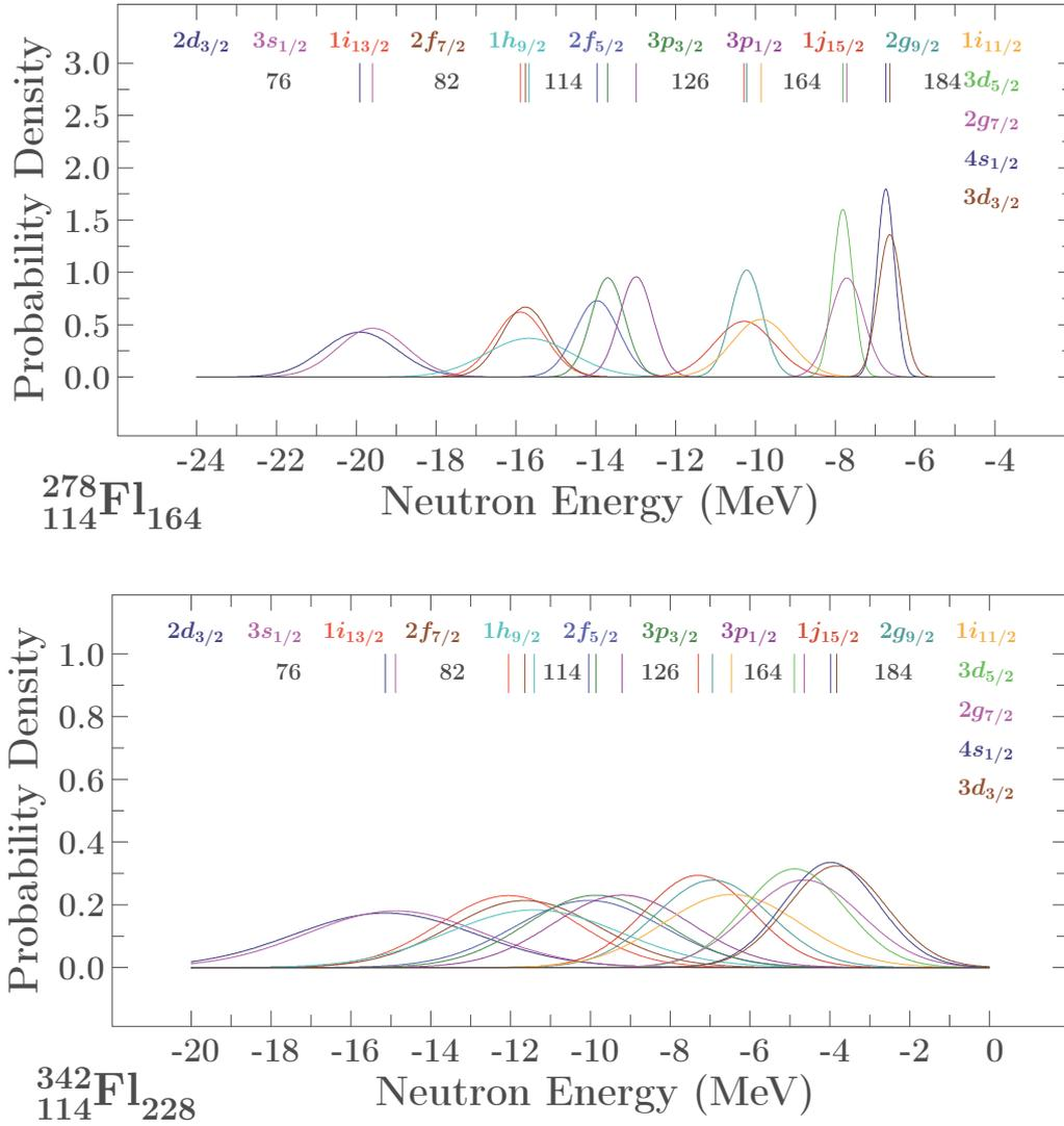
Figure 4.18 – Equivalent to Figure 4.17 but for the  $^{278}\text{Fl}$  super-heavy nucleus (top) and  $^{342}\text{Fl}$  (bottom). The values of the FWHM of each distribution can be found in Table 4.9. Let us emphasise that the distributions are extremely broad, especially for low-lying levels, with FWHM between 4 and 5 MeV in the N=5 shell.
