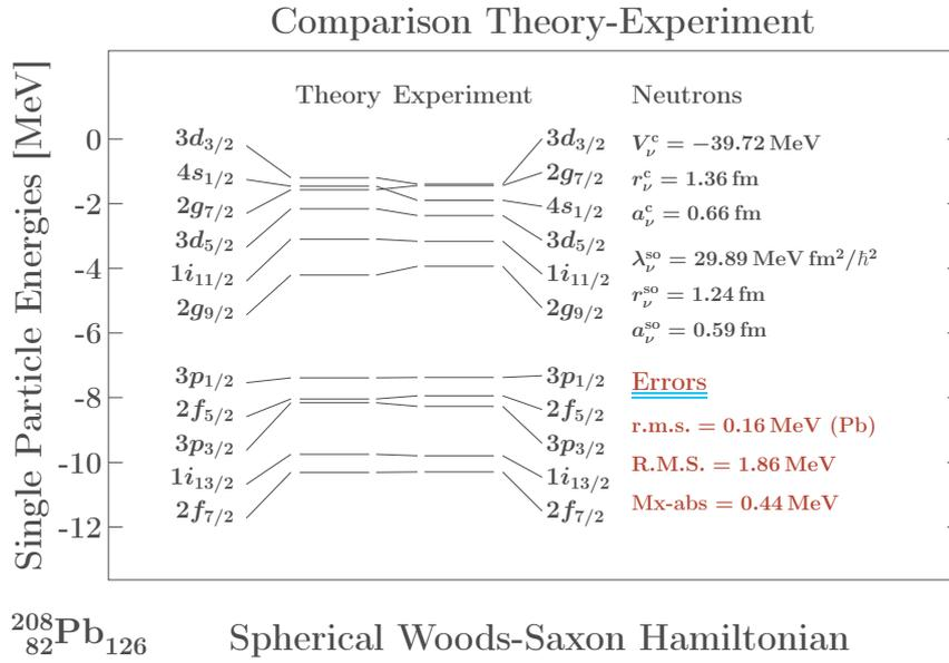
Figure 4.1 – Calculated  $^{208}\text{Pb}$  neutron single particle energies, left column, resulting from the optimisation of parameters of the traditional-WS Hamiltonian. The experimental energies are given in the right column and the parameter values on the right side of the figure. One finds from top to bottom: r.m.s.-deviation from Eq. (3.30), R.M.S.-deviation from Eq. (3.32) and the maximum absolute error, Mx-abs. [Experimental data from Tables 2.2 and 2.3]
