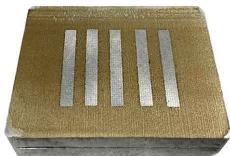
Figure 3.9 Photograph of a thin film soil sample on the surface of an aluminum plate. The visible marks on the sample surface are caused by laser ablation.
