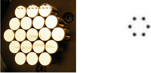
Fig. 11. Left: the active segmented mirror with 19 sub-apertures. Right: Simulation of the parking position in the focal plane with the 6 sub-apertures used (first corona).
