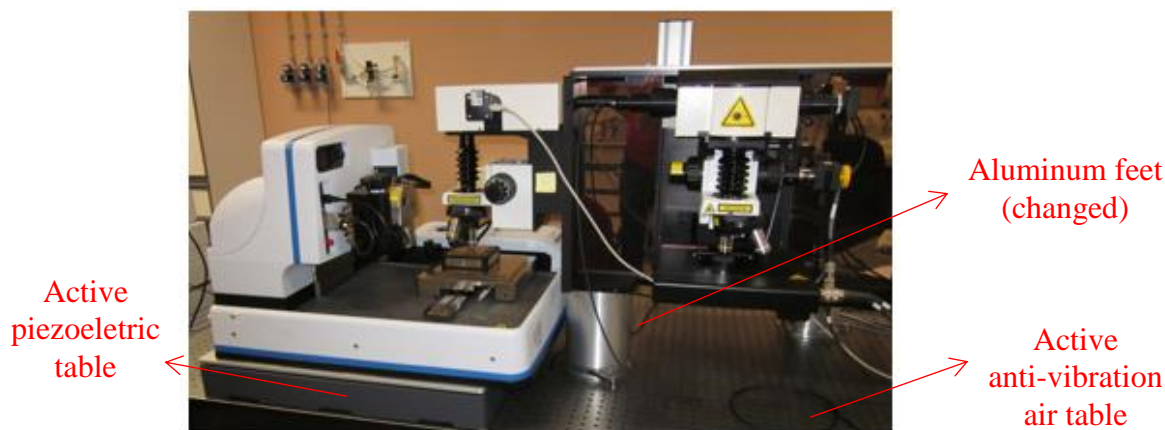
Figure 3.6. Co-localized AFM/Raman setup installed at the laboratory SyMMES
