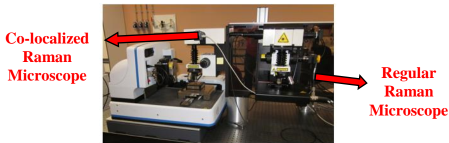
Figure 3.13. Co-localized AFM/Raman setup. The red arrows show the Co-localized Raman Microscope installed in front of the AFM and the Regular Raman Microscope positioned with direct access in front of the user
