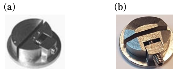
Figure 3.2. Sample holder used to cut thick membranes (a) classical and (b) modified to minimize the risk of collision when cutting thin membranes close to the surface of the holder.
