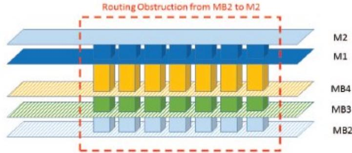
Figure 2.2.1.5 Routing obstruction caused by excess of 3DCO vias in yellow. A connection from the bottom transistor up to M2 in top tier needs vias in all layers between M2 and bottom transistor contact. [Billoint 2015]
