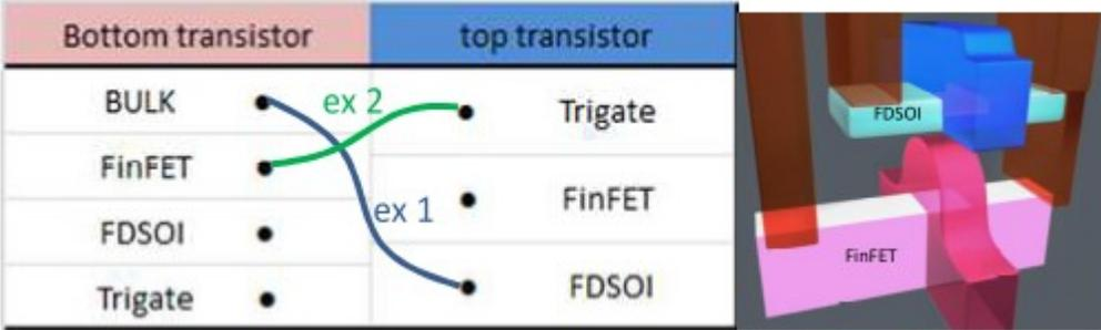
Figure 1.2.3.12 Homogenous 3D integration featuring different transistor architectures in each tier [Batude 2014].
