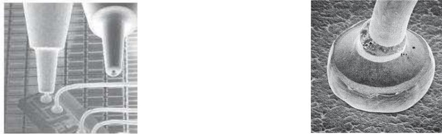
Figure 1-8 – Ball Bonding [K&S Micro-Swiss]
