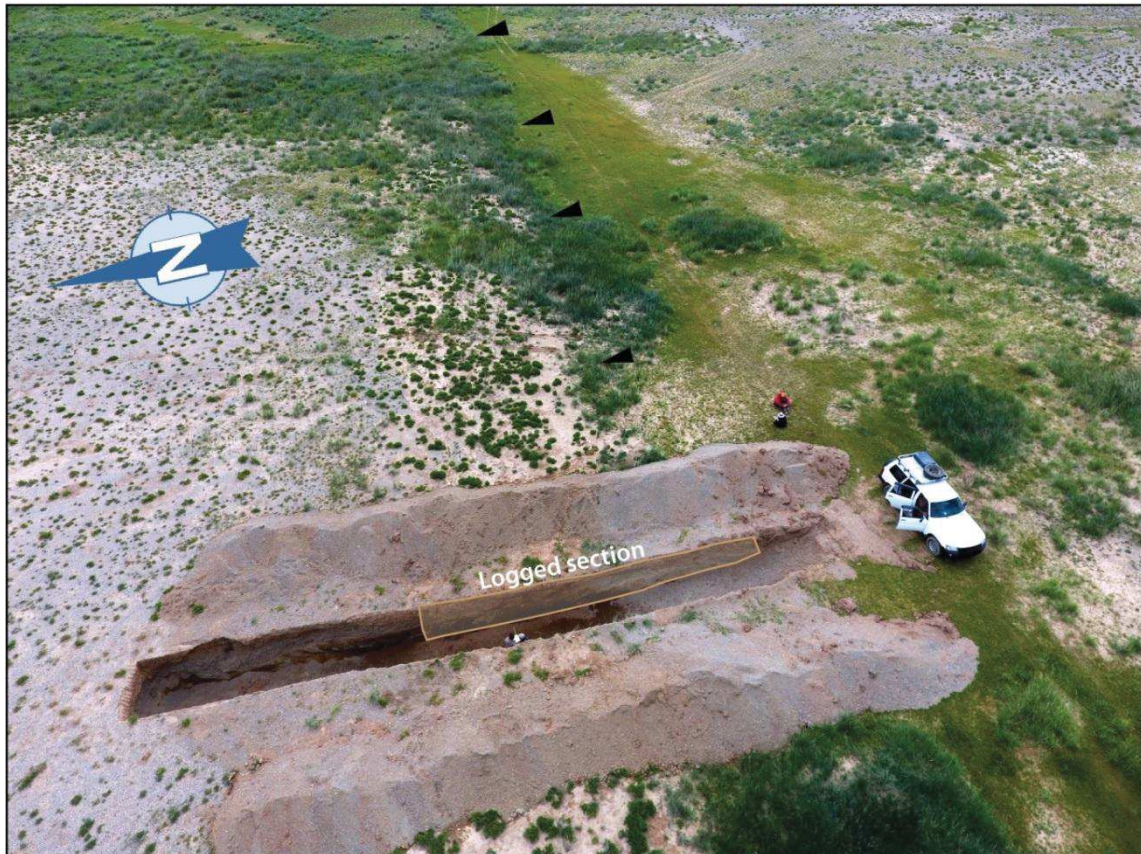
Figure 4-53: Photograph to the East of the Swan Lake Trench. Shaded area is the section of the trench in Figure 4-55. Black arrows indicate the WBF. Note the change of materials when crossing the fault trace.
