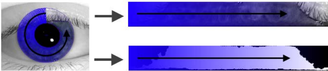
Figure 4: Illustration of the unwrapping process of Daugman's normalization. On the left the segmented image, on the upper right the unwrapped texture of the iris and on the lower right the segmentation mask of the iris region
