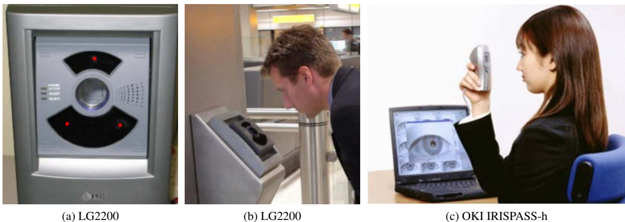
Figure 2: Examples of iris acquisition devices. Figure (a) and (b) : the stop and stare sensor LG2200 from LG with an acquisition range between 8cm - 25cm. Figure (c) : the hand held sensor OKI IRISPASS-h from OKI.
