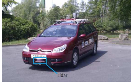
Fig. 2.15: The LIDAR mounted on the experimental vehicle CARMEN in Heudiasyc laboratory.
