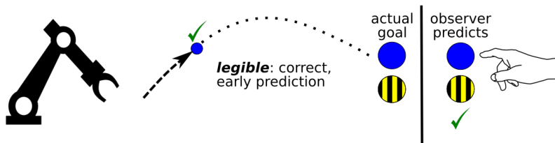
Figure 2.2: Legible motion in a reaching task scenario. This is the most informative type of motion.
