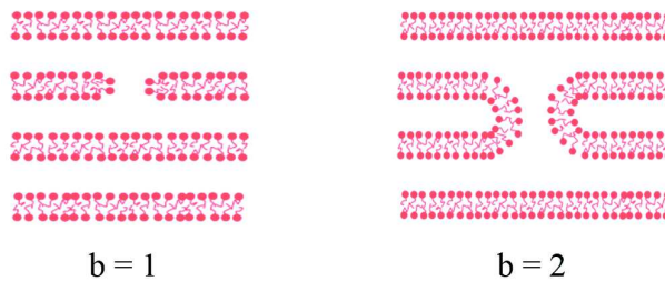
Figure 3.15: Edge dislocations of Burgers vector b = 1 (left) and b = 2 (right) [55]
