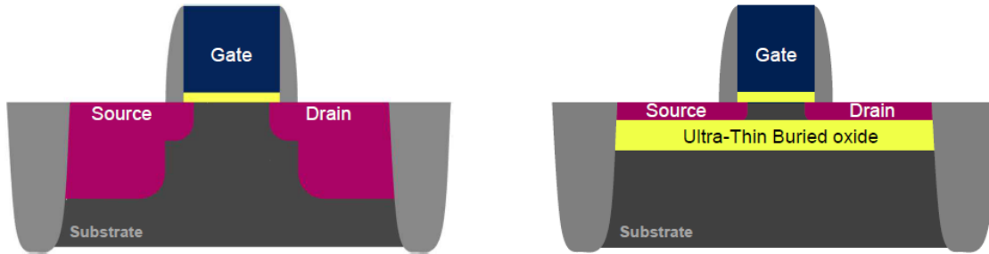
Fig. 3.4: CMOS bulk and FD-SOI transistors cross section.
