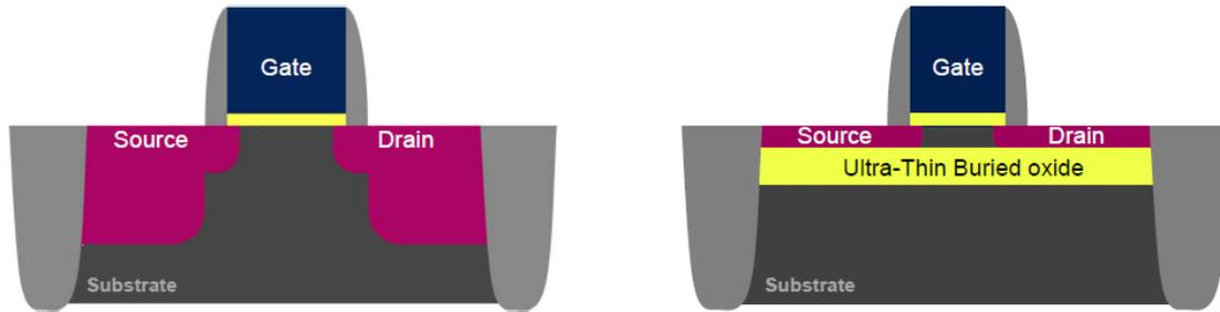
Fig. 3.4: CMOS bulk and FD-SOI transistors cross section.
