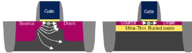
Fig. 1.26: Electron flow in bulk and FD-SOI CMOS transistor.
