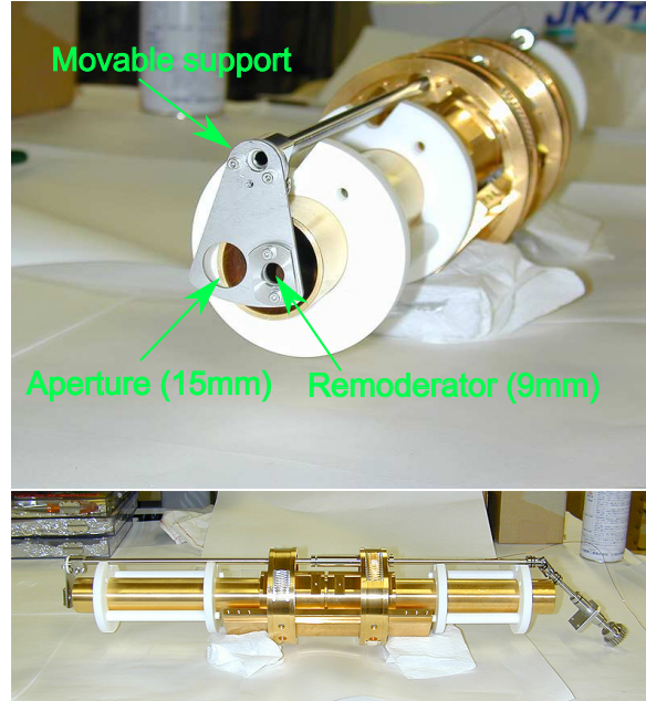
Figure 7.10: One stack of electrodes of the 5 T Penning-Malmberg is shown. The remoderator support is located between two stacks of electrodes and allows the insertion of a remoderator with 9 mm diameter. In order to eject the positrons out of the trap, the support can be moved so that the positrons can pass through a 15 mm aperture.
