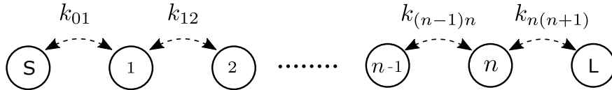
Figure 4.7 – Schematic description of a coupled resonator filter in ladder topology.
