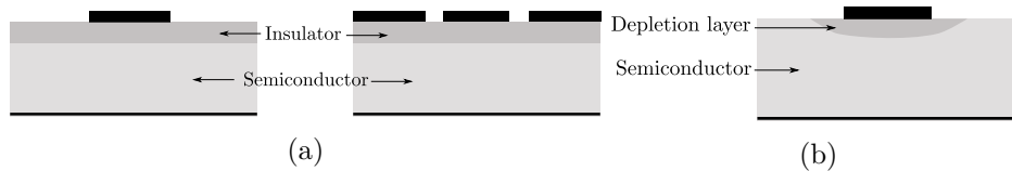
Figure 1.21 – (a) MIS Microstrip and coplanar waveguide (left and right, resp.), (b) Shottky-contact microstrip transmission line.
