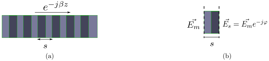
Figure 2.6 – Principle of the eigen-mode simulation: (a) Periodic waveguide, (b) equivalent resonant unit-cell.
