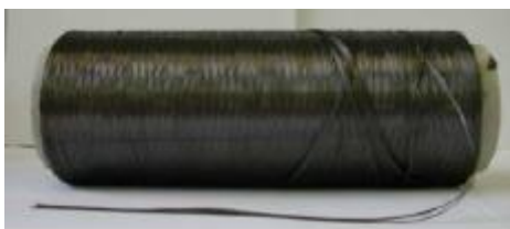
Figure 4.1 Carbon fiber bobbin. The roving is of a bundle of parallel strands without twisting. Picture adapted from Cong Lu thesis, Electrochimie UMR 8640.
