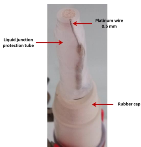
Figure 4.6 Platinum wire and rubber cap placed over the liquid junction protection tube.
