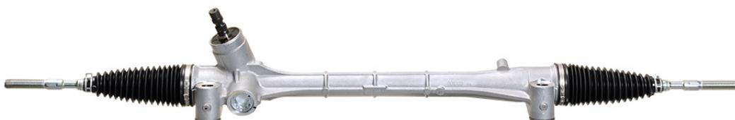
Figure II.3 – Manual Steering System
