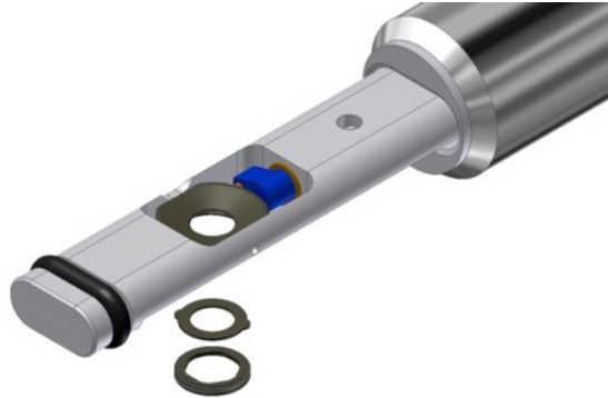
Fig. II.5: Schematic representation of the head of a vacuum transfer holder for FEI microscopes. After loading a TEM grid, the head can retract and hermetically seal the sample from ambient conditions.
