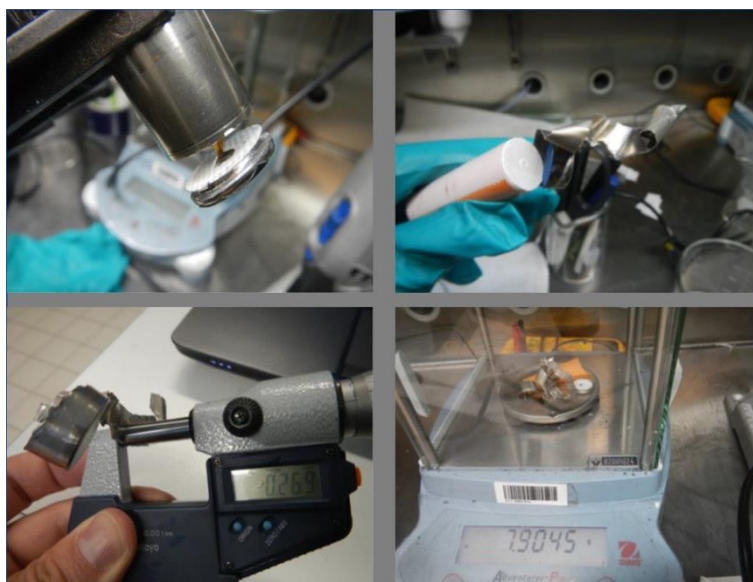
Figure 47 – The cutting sequence with the successive measures of the casing thickness and weight are reported from the upper-left picture in clockwise order.
