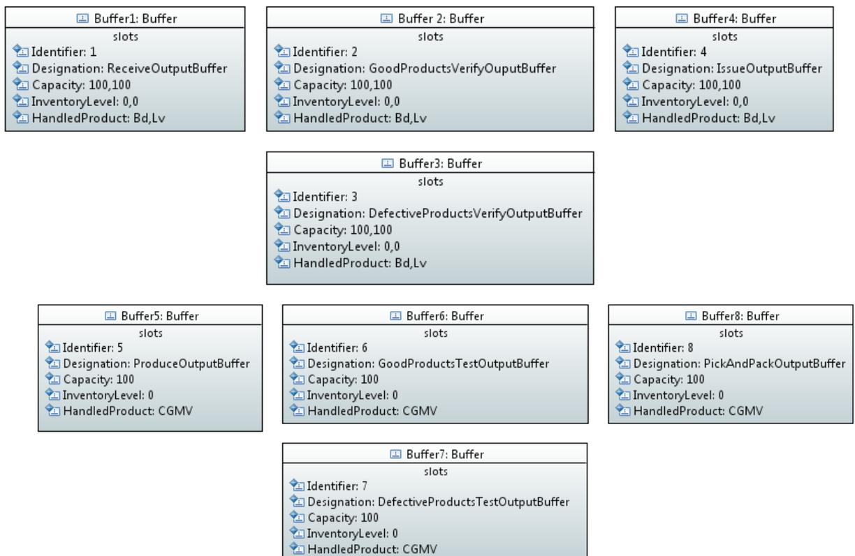
FIGURE A4.16: THE BUFFER INSTANCE BELONGING TO GTM FACILITY
