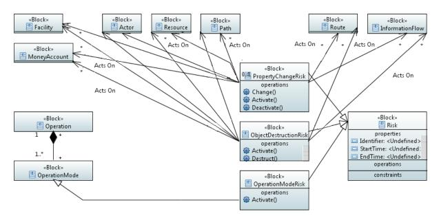
Figure 3.20: SC risk meta-model block definition diagram
