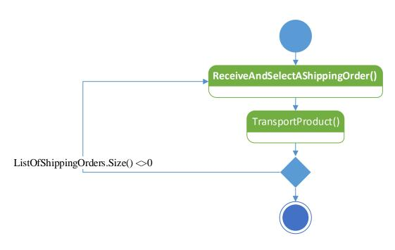
FIGURE A1.15: THE STATE MACHINE OF THE SHIPPRODUCT OPERATION
