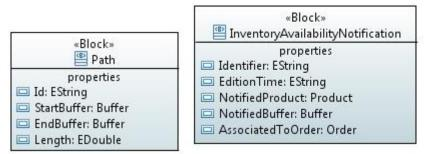
FIGURE A1.23: DETAILS OF THE USED IMPUTS AND OUTPUTS FOR THE TRANSFER OPERATION
