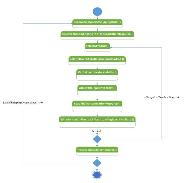
FIGURE A1.12: THE STATE MACHINE OF THE ALGORITHM OF THE LOADVEHICLE OPERATION
