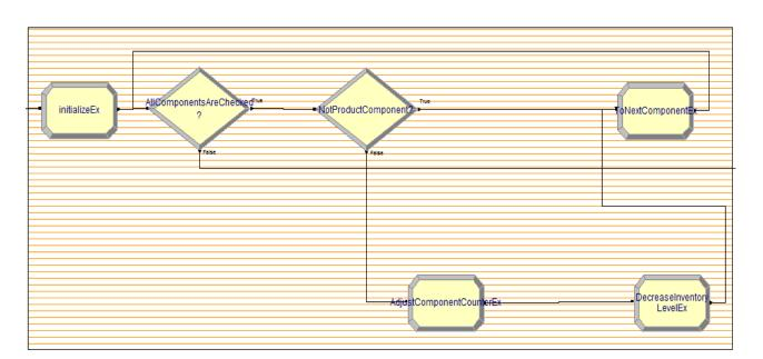
FIGURE 4.6: FLOWCHART OF THE CONSUMECOMPONENTS () METHOD ARENA SUBMODEL
