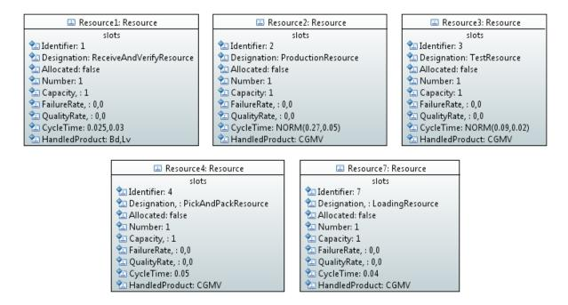
FIGURE A4.11: THE RESOURCE INSTANCES DIAGRAM BELONGING TO GTM FACILITY
