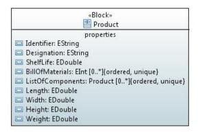
FIGURE 3.5: THE PRODUCT VIEW BLOCK DEFINITION DIAGRAM
