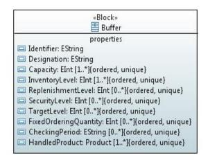
FIGURE 4.2: THE TRANSLATED BUFFER CONSTRUCT
