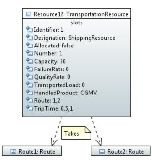
Figure 5.9: Example of an instance of the Transportation Resource used for shipping to DistC1 and DistC2 facilities
