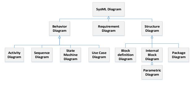
Figure 2.2: The SysML diagrams (Adapted from  $\text{omgSysml}^2$ )
