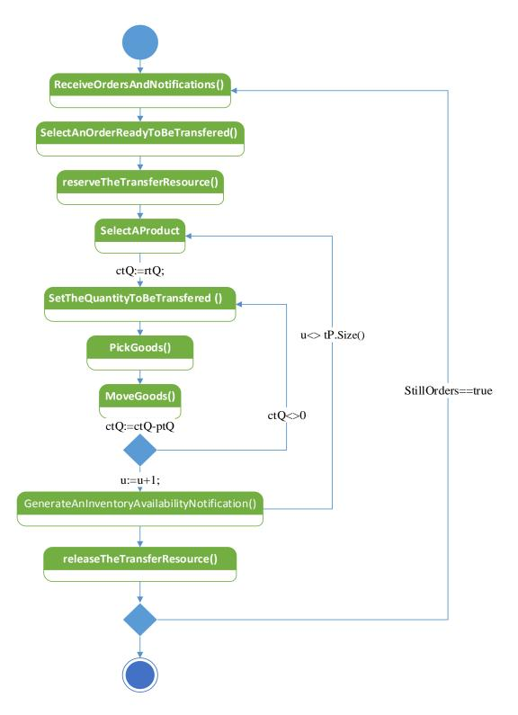
FIGURE A1.24: THE STATE MACHINE OF THE TRANSFER OPERATION
