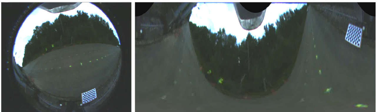
Fig. 3.5: Intrinsic calibration: qualitative verification by undistorting the image into a panoramic image
