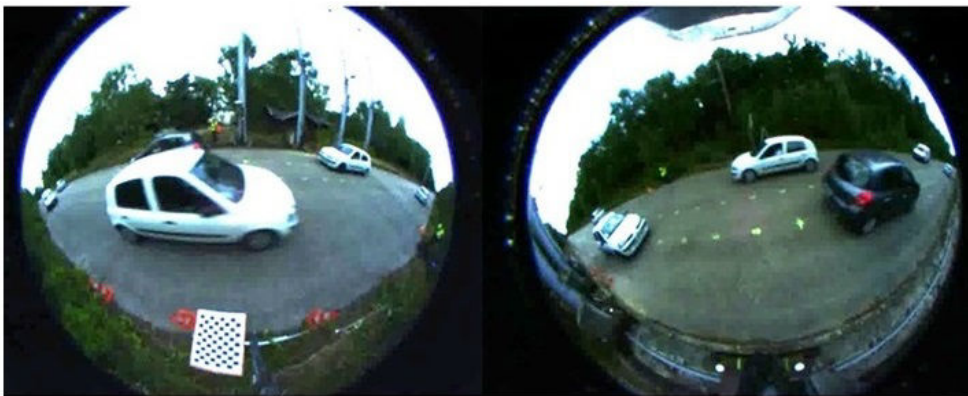
Fig. 3.6: Introducing the fisheye-stereo monitoring system - Lab dataset: note how the occluded black car in the left image is fully visible in the right image; multi-view data association is also a major issue
