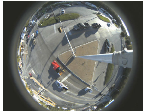
Fig. 2.13: Example view from a fish-eye camera in the center of an intersection [88]
