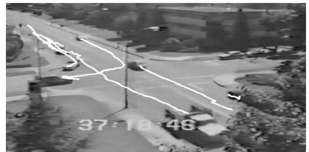
Fig. 2.16: A feature-based vehicle tracking at intersections [149] (2006)
