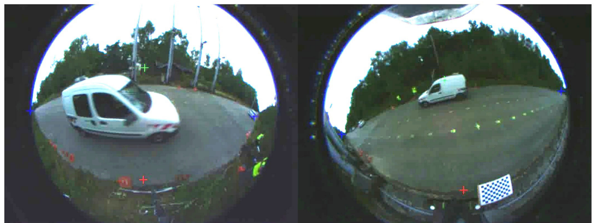
Fig. 3.14: Orthogonal trihedron of vanishing point estimation approach. a) great circles normals from trajectories are retro-projected in the fisheye image (yellow), the reprojection of VP_1 is represented in blue. b) location of vanishing points hypothesis, VP_2 (green) and VP_3 (red). c) the complete solution ( VP_2 - green ; VP_1 - blue ; VP_3 - red).
