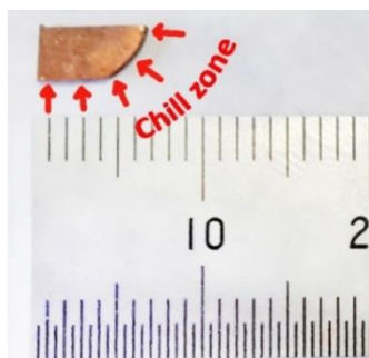
Figure III.1. A photograph of an as-cast \text{Cu}_{90}\text{Zr}_5\text{Hf}_5 sample fragment, with an indication of the chill-zone localization.
