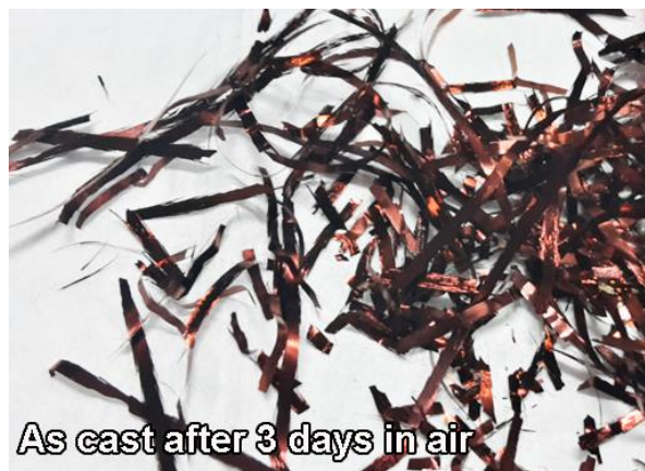
Figure III.10. A photograph of a Cu-Ca melt-spun ribbon 3 days since casting.
