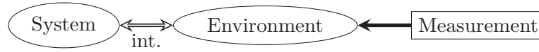
Figure 4.2: Typical mesoscopic physics lab experiment: a solid state quantum device is never accessed directly but through measurements performed in its electromagnetic environment part of which consists in coaxial cables extracting and bringing microwave radiation to the device.
