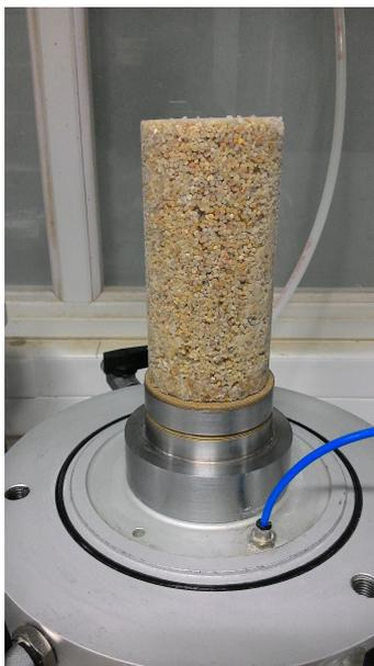
Figure 4.14: Frozen eroded specimen prepared for triaxial compression test.
