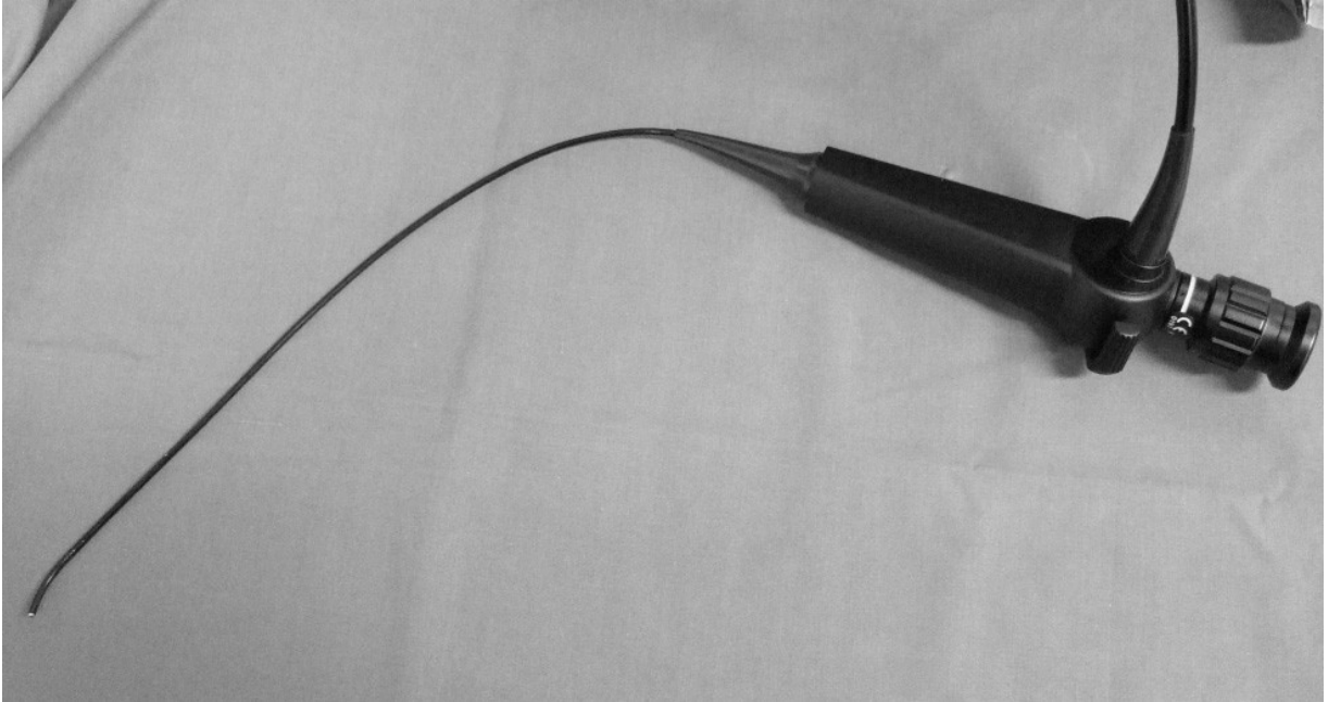
Figure 1.5: Flexible Endoscope for Vocal Cords' Inspection [19]
