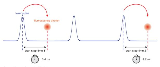
**Figure 14 Principle of TCSPC**
