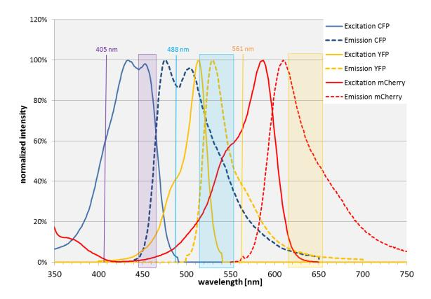
Figure 13 Laser excitation and emission detection of the Partec Flow Cytometer
