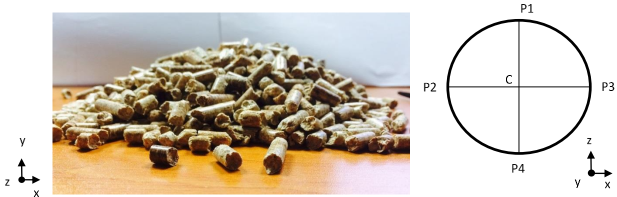
Figure I.5: Static angle of repose for pellets (left) and schematic of measurement points P1, P2, P3 and P4 with the center point C (right)
