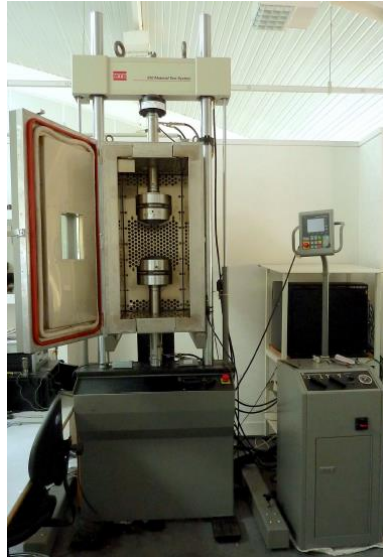
Figure 24. MTS 810 servo-hydraulic testing machine
