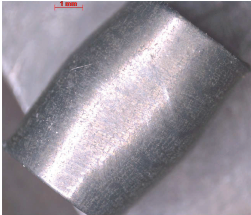
Fig. A6-2 - VCG SHE compression creep specimen tested under 750°C/- 800 MPa
