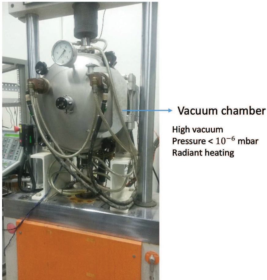
Figure 2.14 - Servohydraulic Instron 1271 testing system with a high vacuum chamber.
