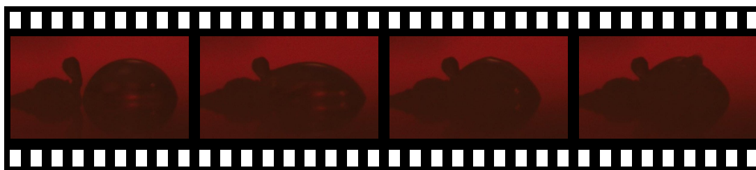
Figure 86: Substrate seen from the side camera. Many drops are sent at the same place on a substrate of PDMS at 17^{\circ}\text{C} at 100 Hz, close to pieces of frozen hexanediol. For the first 70 s, the drops remain liquid and form an increasingly large drop, as seen on the first picture. On the second picture, 0.2 s later, the drop touches the frozen ink and spreads on it. On the third picture, 2.8 s later, a freezing front is clearly visible. Finally, in the fourth picture, after 0.6 s, the hexanediol is completely solid and the next drops start to form a column on the right of the frozen drop. This abrupt freezing is a clear signature of the existence of a supercooled phase.
