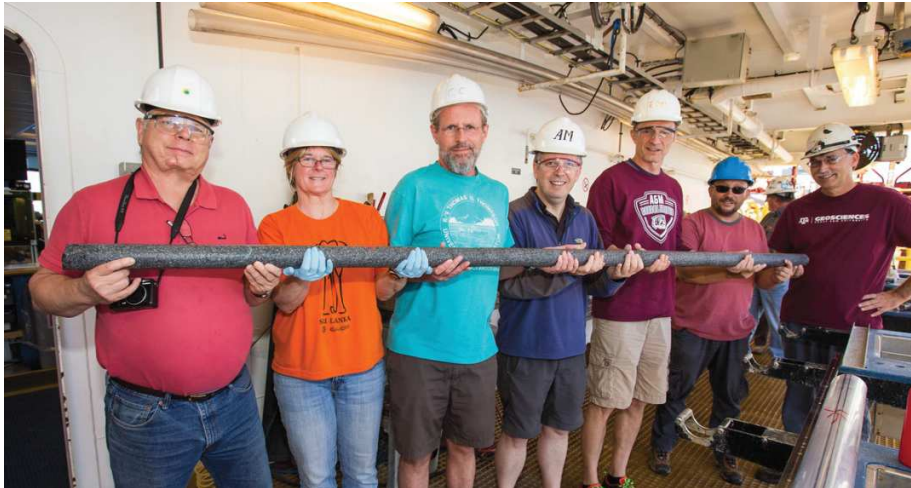
Figure IV.6 - Longest piece (2.85 m) of rock recovered in core 66R at 603 mbsf during Expedition 360 at the Atlantis Bank (MacLeod et al. , 2017b).
