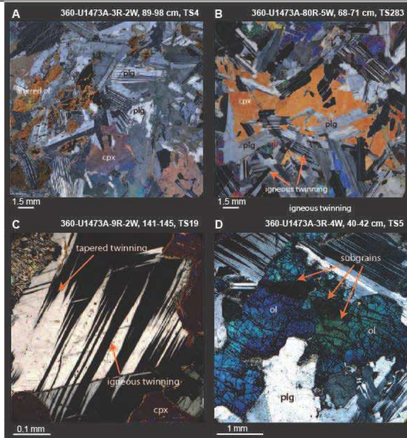
Figure IV.14 – Characteristic textures of gabbros from Hole U1473A: a) euhedral randomly oriented elongated and tabular plagioclase (Pl) showing igneous and tapered twins (3R-2, 89–98 cm; XPL). Clinopyroxene (Cpx) is subophitic and undeformed; b) weakly developed preferred dimensional orientation of tabular elongated Pl showing igneous twinning with undeformed Cpx oikocryst including Pl chadacrysts (80R-5, 68–71 cm; XPL). c) preserved and slightly bent igneous twins and tapered twins in Pl (9R-2, 141–145 cm; XPL); d) deformed olivine (Ol) grain displaying straight subgrain boundaries (3R-4, 40–42 cm; XPL)
