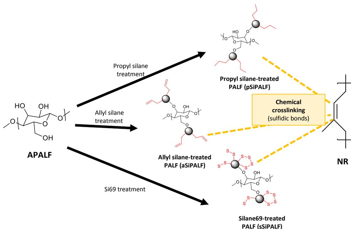
**Figure 5.20** The reaction schemes of silane treatments
