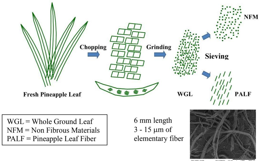
**Figure 3.23** Extraction of PALF at Mahidol University [63]
