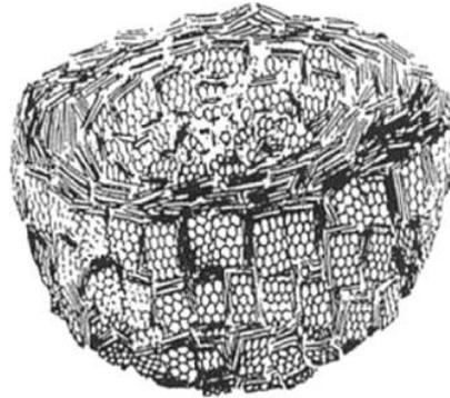
**Figure 3.17** Sketch of carbon black primary particle [49]
