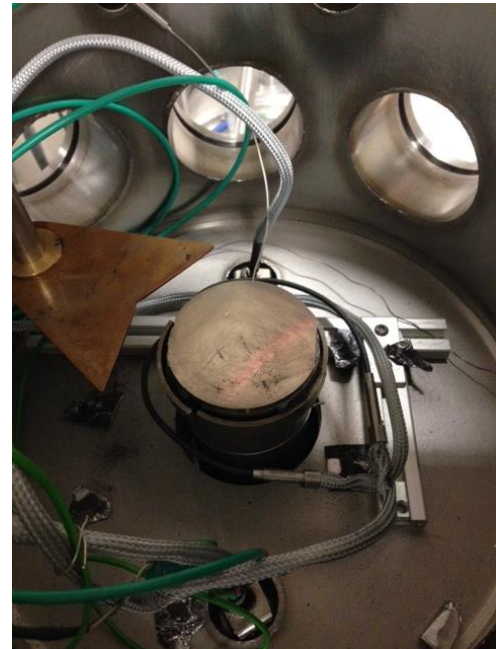
Figure 2.4.2: Picture of the Inconel bottom clamp in the vacuum chamber. Heating resistances are supplied by armoured cables. Copper plate sample holder allow to process multiple samples without opening the chamber.
