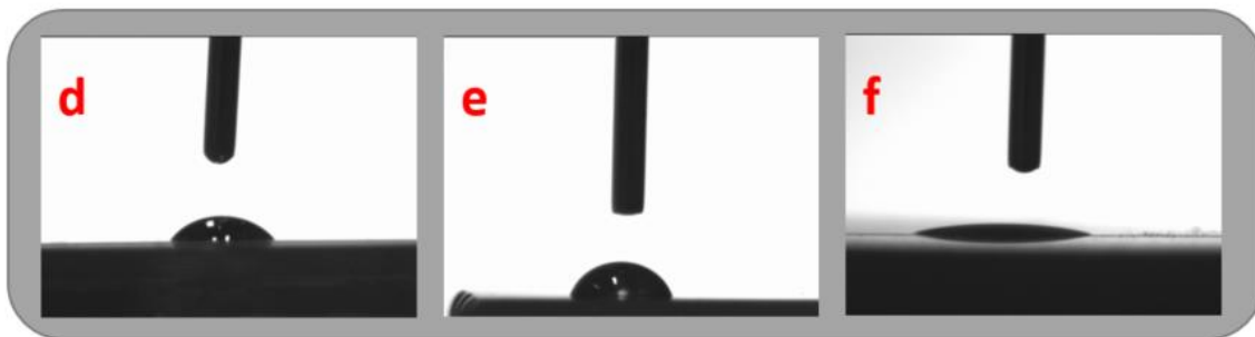
Figure 4.5.3 : Images of diiodomethane droplets deposited on Zr3 surfaces after 60 seconds for 1\ \mu\text{m} polished surface (d), LIPSS texture surface (e) and Ridge texture surface (f) tip of the syringe is 0.8 mm in diameter.
