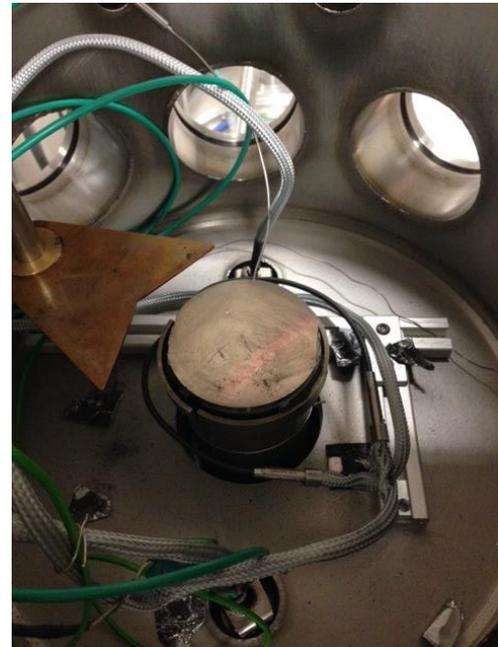
Figure 2.4.2: Picture of the Inconel bottom clamp in the vacuum chamber. Heating resistances are supplied by armored cables. Copper plate sample holder allow to process multiple samples without opening the chamber.
