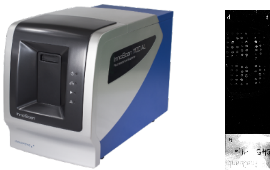
Figure 1.2: From left to right: the scanner named InnoScan 1100 AL (source: https://www.innopsys.com/ ) and a fluorescence TMA image scanned using this device (by the courtesy of Innopsys).
