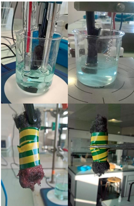
Figure 7-5: Voltammetry tests (a), electrowinning experiments, carbon felt cathode after (c) and before deposition (d).
