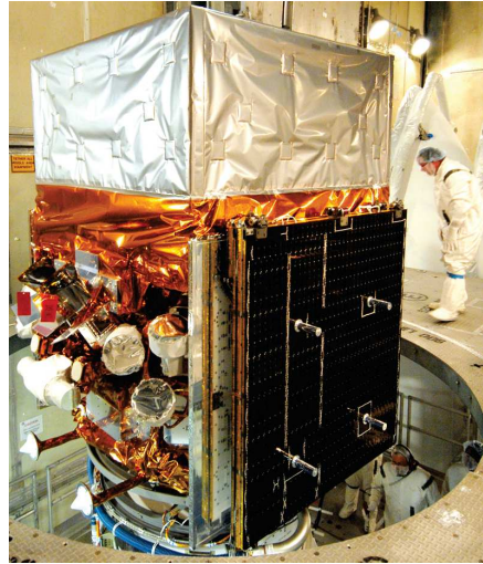
Figure 2.1: The Fermi spacecraft and its payload: the LAT instrument at the top is here covered by its anti-meteorite shield, while the GBM scintillators are visible at the bottom (left) side.
