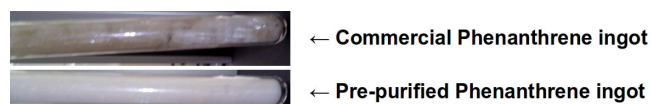
FIG. 35: Pictures of Phenanthrene ingots without and with application of the pre-purification procedure
