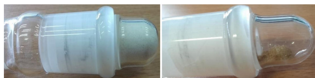
FIG. 45: Pictures of the sample holder before (left) and after (right) the sublimation experiment
