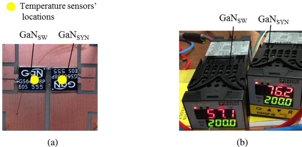
**Fig. 3-16:** Temperature sensor location (a) and PID regulator screen (b)
