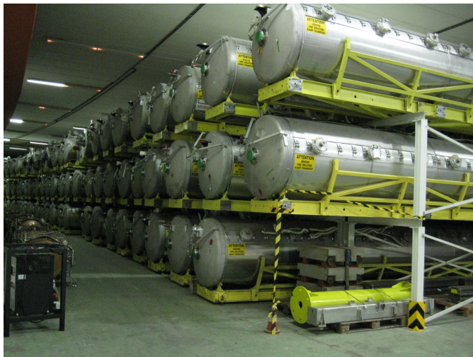
Figure 2.2: An example of waste family produced and stored at CERN. These metallic elements are accelerating cavities of the LEP machine.
