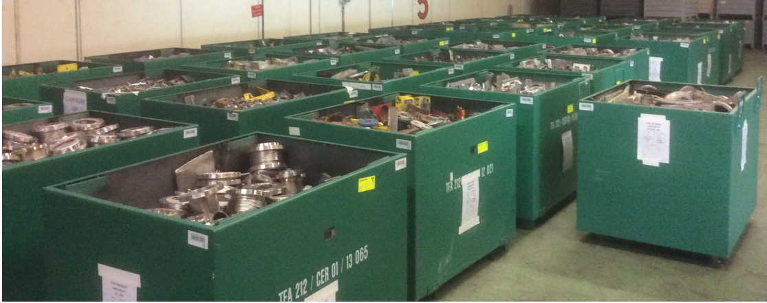
Figure 3.4: A batch of 1.3 m 3 packages containing metallic VLLW. Credits: B. Cellier, CERN.
