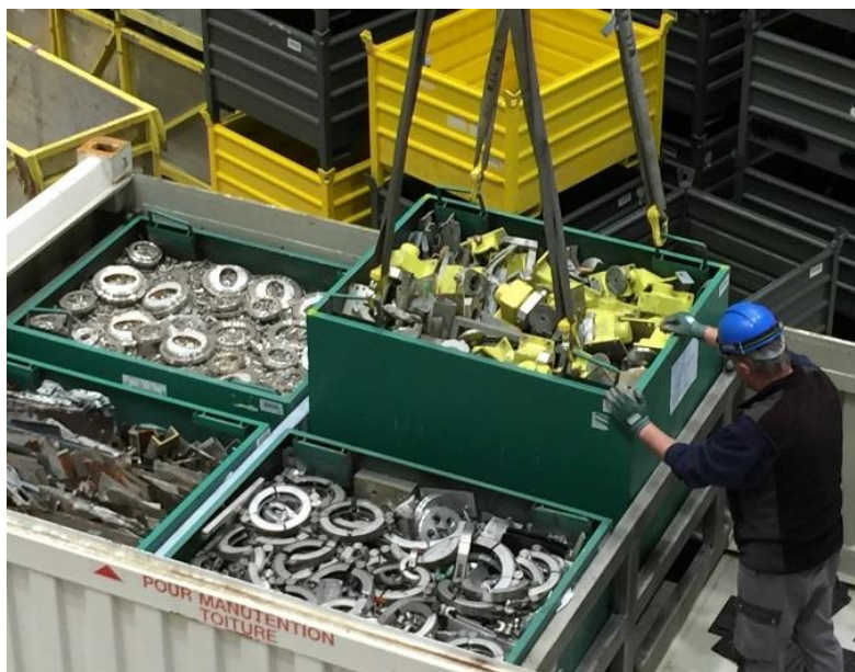
Figure 5.14: Loading of standard packages filled with metallic VLLW ready for transport to the ANDRA disposal facility [Bruno et al. 2017].
