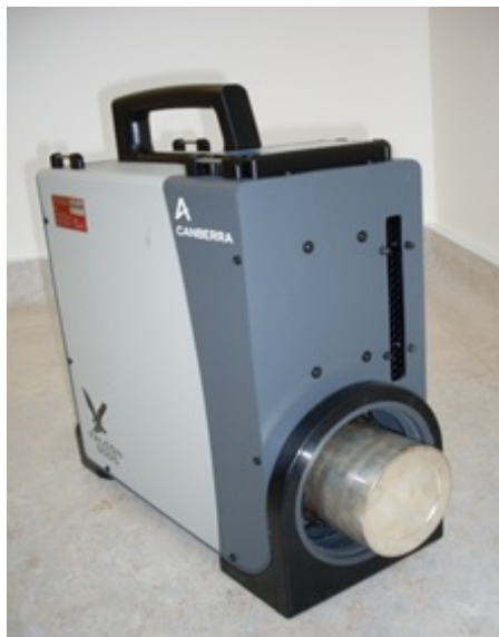
Figure 3.2: Falcon5k is an electrically chilled and portable \gamma -ray detector. This system is commonly used at CERN to quantify the activity of ETM radionuclides in radioactive waste.
