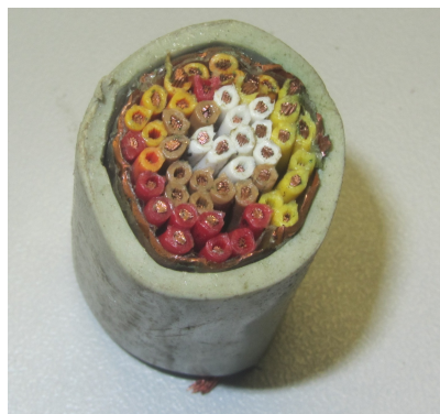
Figure 5.2: Sample CR-049985 of copper signal cable ( \phi = 2\text{cm} ). Photo credit: F.P. La Torre, CERN.
