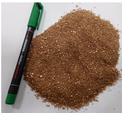
Figure 5.4: Example of shredded copper.
