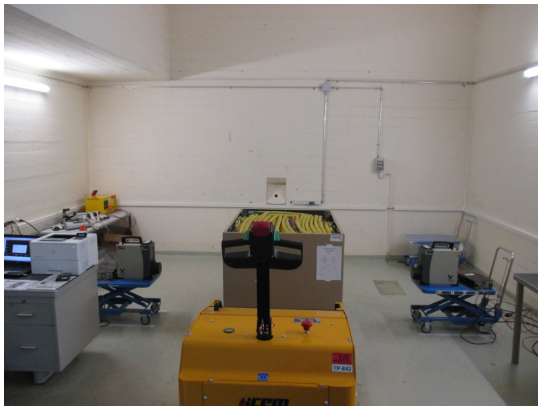
Figure 5.15: Spectrometric measurement system deployed at CERN for the measurement of ETM radionuclides [Bruno et al. 2017].
