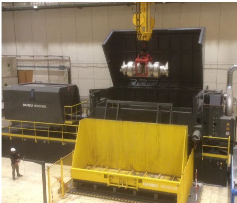
Figure 5.12: Processing of a radioactive waste item by the press-shears [Bruno et al. 2017].
