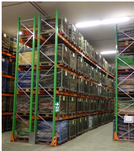
Figure 2.3: An example of activated cables produced at CERN, presently being disposed of as VLLW.
