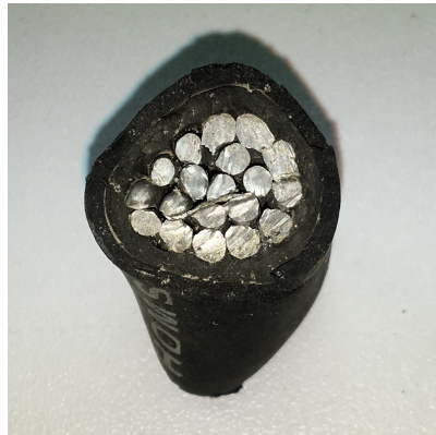
Figure 5.1: Sample CR-049963 of aluminium power cable ( \phi = 1.8\text{cm} ). Photo credit: F.P. La Torre, CERN.
