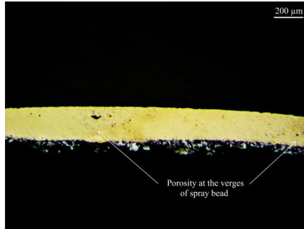
Fig. 86 Cu3 coating on PA6 with Sn+Al 2 O 3 interlayer (light microscope)
